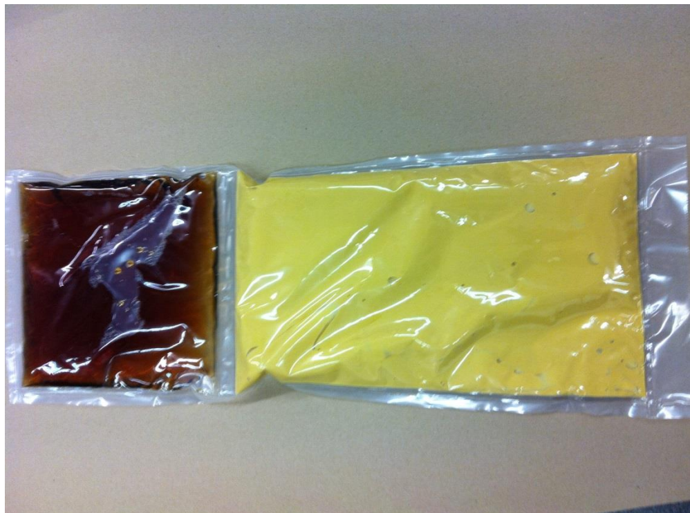
Figure 1. Bag with the separated two compound polyurethane resin ( peelable seal)
