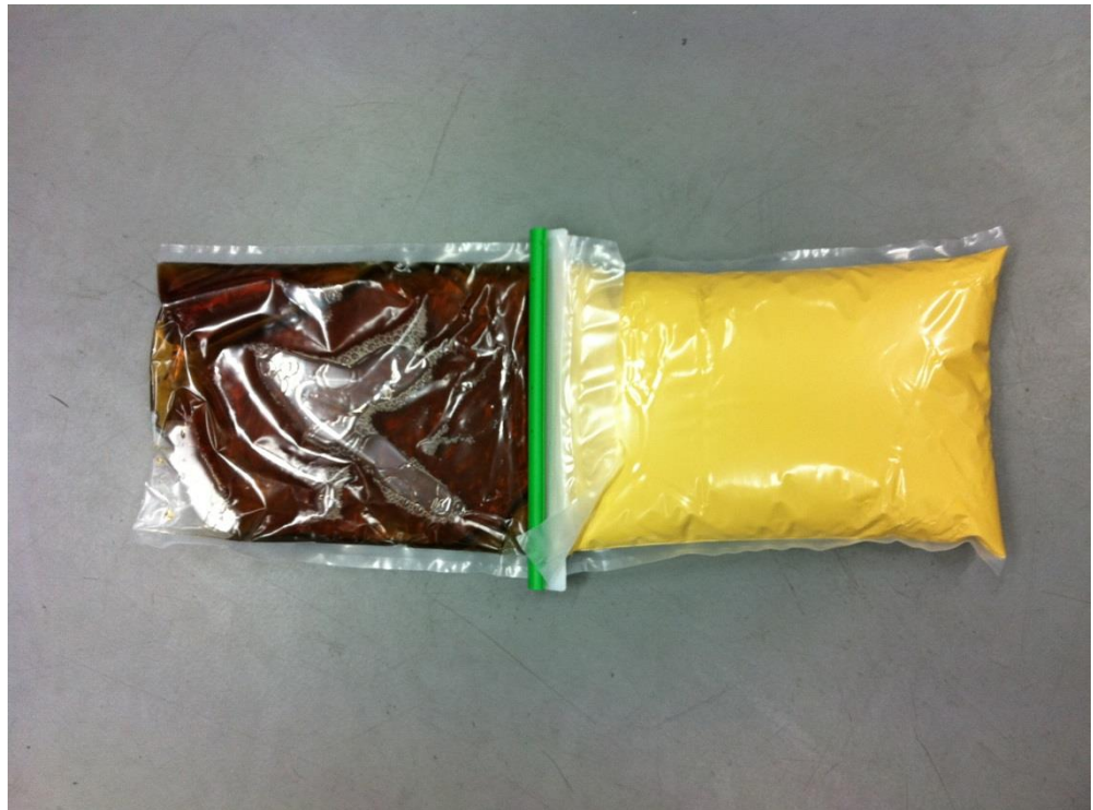
Figure 3. Bag with the separated two compound polyurethane resin ( Pouch Clip)
